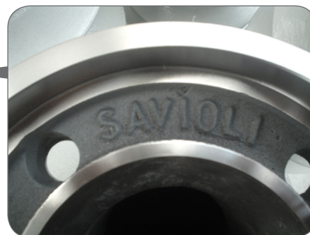
Centering ring integrated in screw casting
